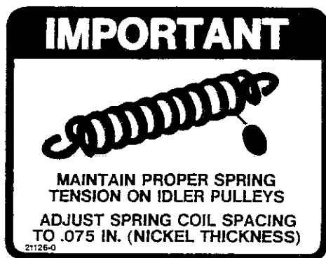
FIGURE 3 - SPRING ADJUSTMENT
